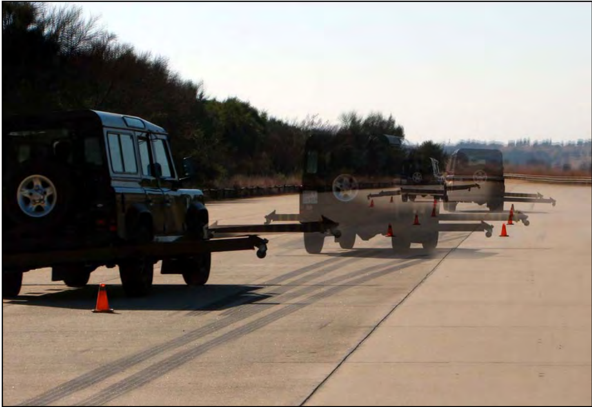
Figure 5.2: DLC manoeuvre sequence.
