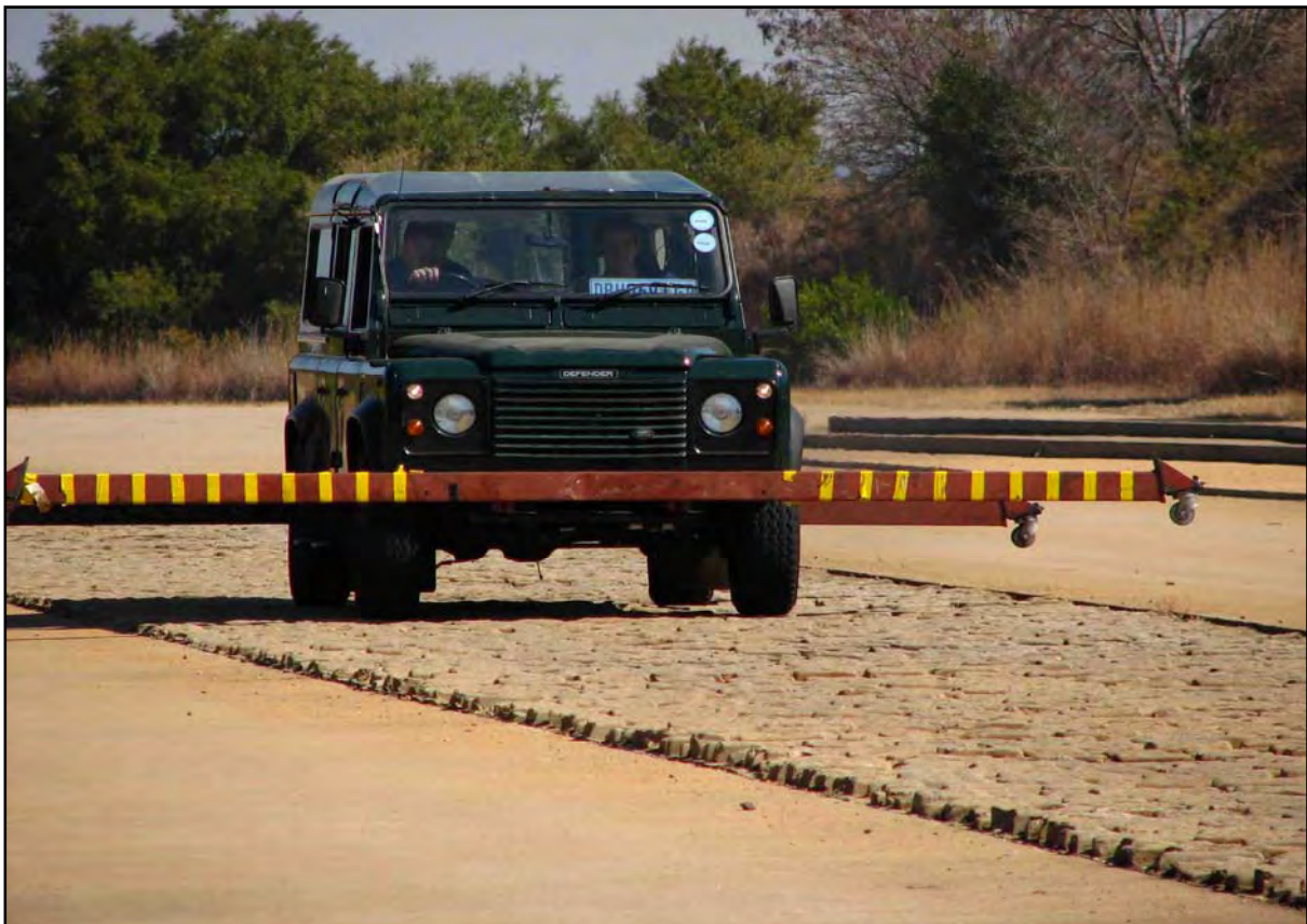
Figure 5.3: Belgian paving test run.
