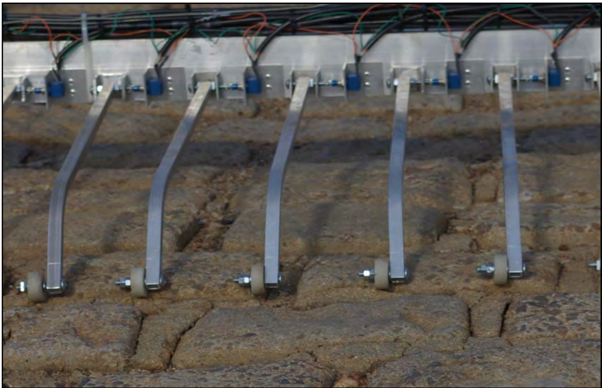
Figure 3.10: Fingers measuring the surface profile of the Belgian paving (Becker, 2008).
