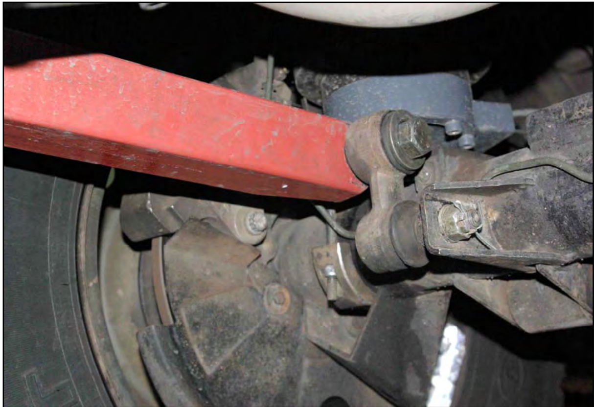
Figure 4.11: AARB fastened on the left hand side to the rear axle.
